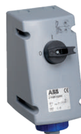
Vertical, Type MVS...W 16 A...32 A, IP67
