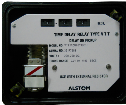
Type VTT with cover removed
